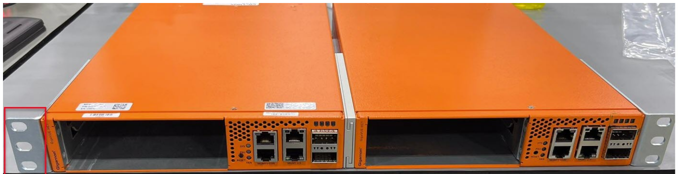
Rack ears face towards the front of the node for Front mounting
